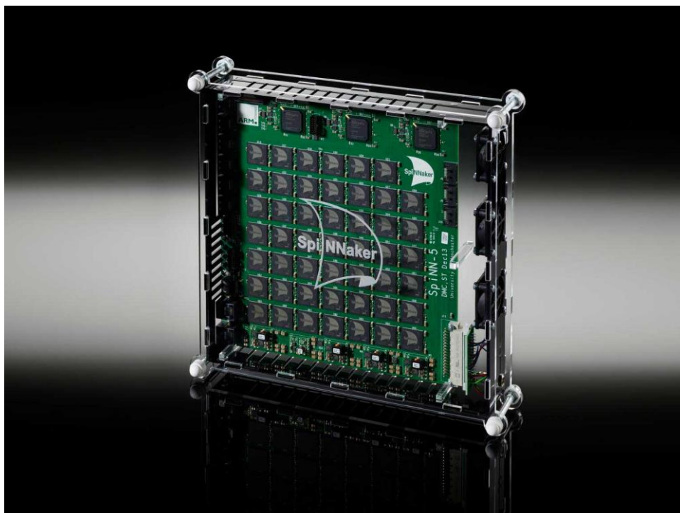
Figure 8 A 48-node SpiNNaker board, release in 2011, consists of 48 nodes each containing 18 ARM 968 cores and proprietary routing technology
